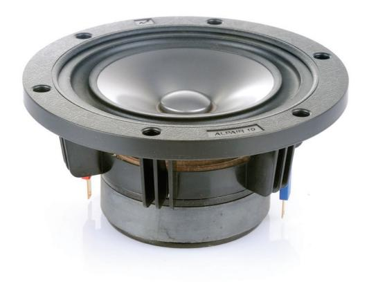
This Alpair 10 Gen.3 is the latest model in a development line designed to extend the performance of mid-sized Markaudio full-range emitters. This generation of Alpair 10 utilises a new ultra thin wall coil. Together with a further modifications to the cone, this latest model delivers usable frequency range up to 25-kHz while retaining its "purist" single cone design,
