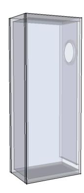
o/ drawing uses 3/4" (19.1mm) material. 18-20mm OK. Quality multi-ply recommended 1/ stuff with 0.75 lbs / ft^3 (1.59 pounds = 0.72 kg) of polyfill 2/cleats on back to allow for removable back, useful for adjusting the stuffing
