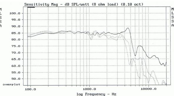
Measured on IEC baffle using Bruel & Kjaer 3144 model microphone. Sensitivity Mag at 0°, 30°, 45°
